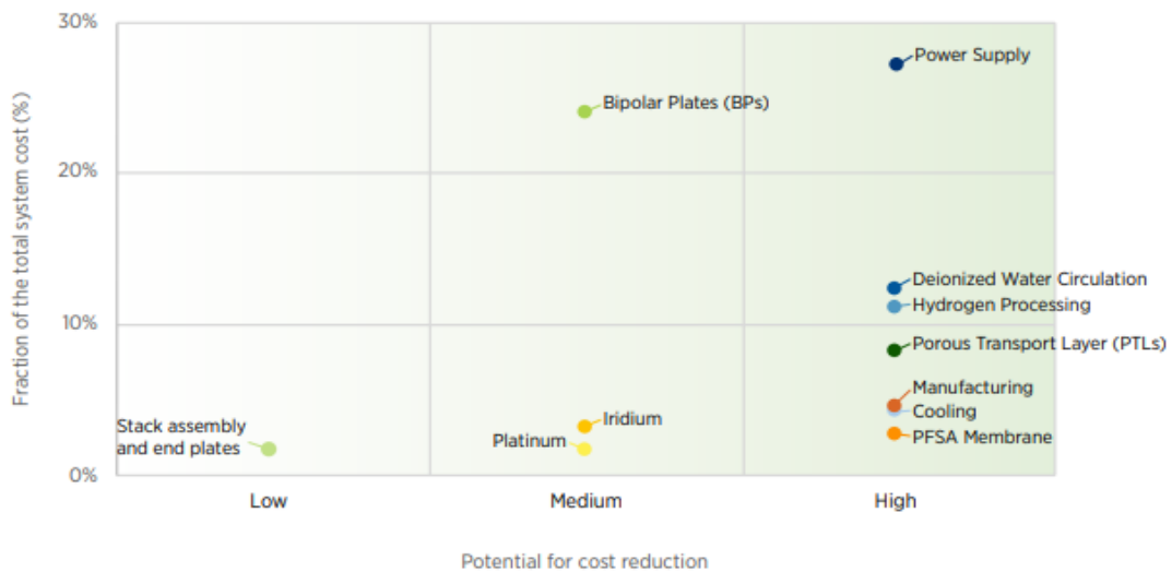
Figure 19. System components for a 1 MW PEM electrolyser classified based on contribution to total system cost and potential for cost reduction.
